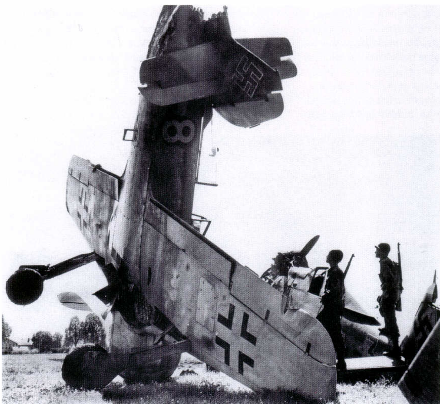
337: An unusually finished Fw 190A-3, WNr 2168, 'White 8', which has somehow survived until 1945. Found with many other wrecks at Bad Aibling, it has apparently been completely refinished in late-war style markings and finishes. While the upper surface pattern is probably in 74/75, the underside of the fuselage appears to be unpainted, while the wings are heavily worn 76. Why so much effort should have been expended on what was effectively an obsolescent aircraft is a mystery. Possibly it was meant for use as a Mistel component
