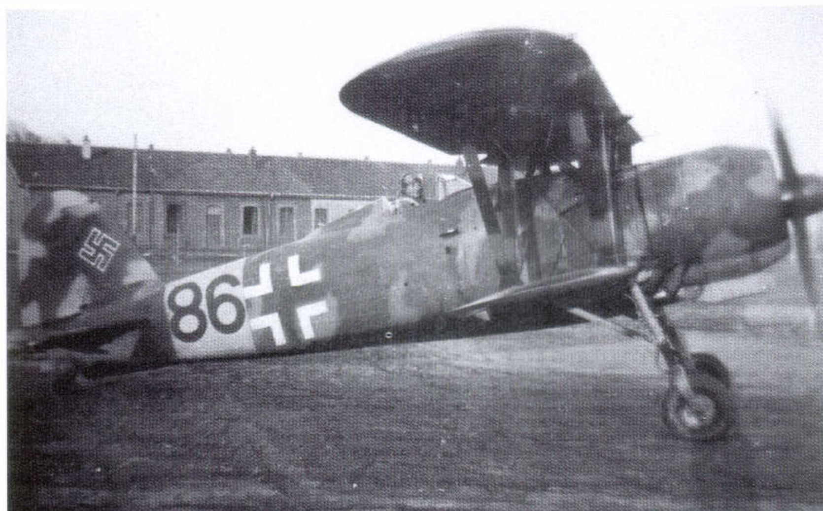
130: As the war progressed many unusual aircraft were press-ganged into Luftwaffe service, among them this Fiat CR 42 used for training. Camouflage on 'Black 86' is RLM 71 with 02 blotches and an 04 Gelb band. The national markings are of the late-war maximum simplified type. Note that the wheel fairings have been removed to simplify maintenance
