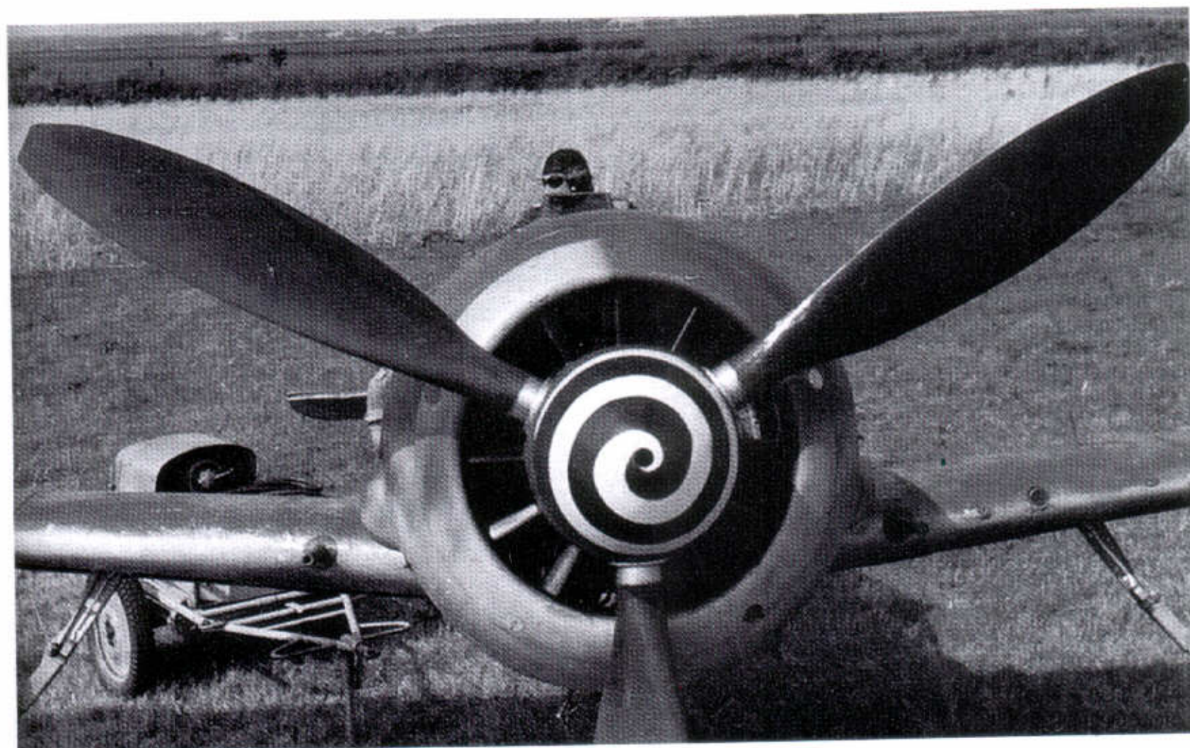
367: A superb view of the engine and propeller of an Fw 190A which clearly shows the 30mm unpainted section at the root of each blade to allow checking for blade adjustment (see page 247). It also shows the white spiral on the black painted spinner. This was in accordance with the order of 10 February 1944 which stipulated that all fighter aircraft of Luftflotte 3 and Luftflotte Reich were to have such a marking. See page 173
