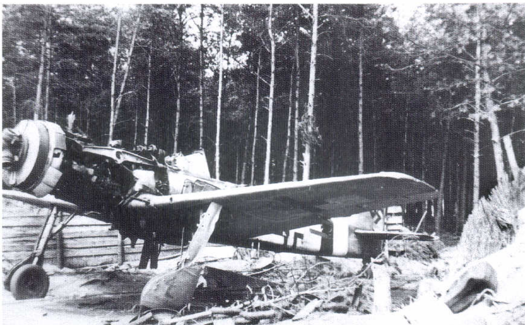
124: This Fw 190D, WNr 211164, 'Black chevron 4' was abandoned at Prague-Ruzyně at the end of the war. Once of the Stab of JG 2 or JG 6, it exhibits a variety of finishes. The fuselage sides appear to be a very pale version of RLM 76, with what may be RLM 82 on top of the engine cowling. The dark tone of the undercarriage fairing suggests that it is in weathered unpainted metal, as was demanded on aircraft produced late in the war. (See page 183). Note that the maintenance instructions have still been applied to the leg fairing. National markings are strictly as the regulations
