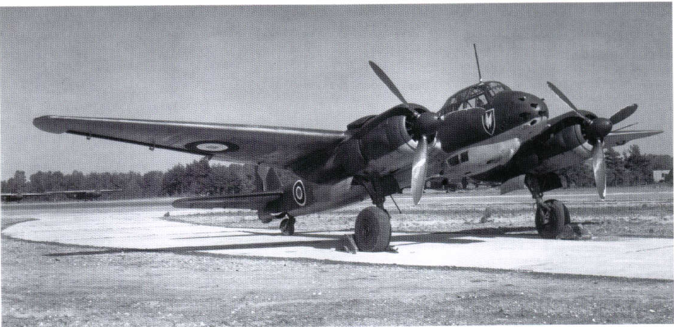
234 Above: Ju 88R-1, WNr 360043, D5+EV, in British markings. The aircraft has a 70/71/65 finish with over-painted German markings. The sharp colour demarcations line between the 65 and the upper camouflage colors is a sign of careful application of the paint, giving the expensive aircraft very good surface protection
