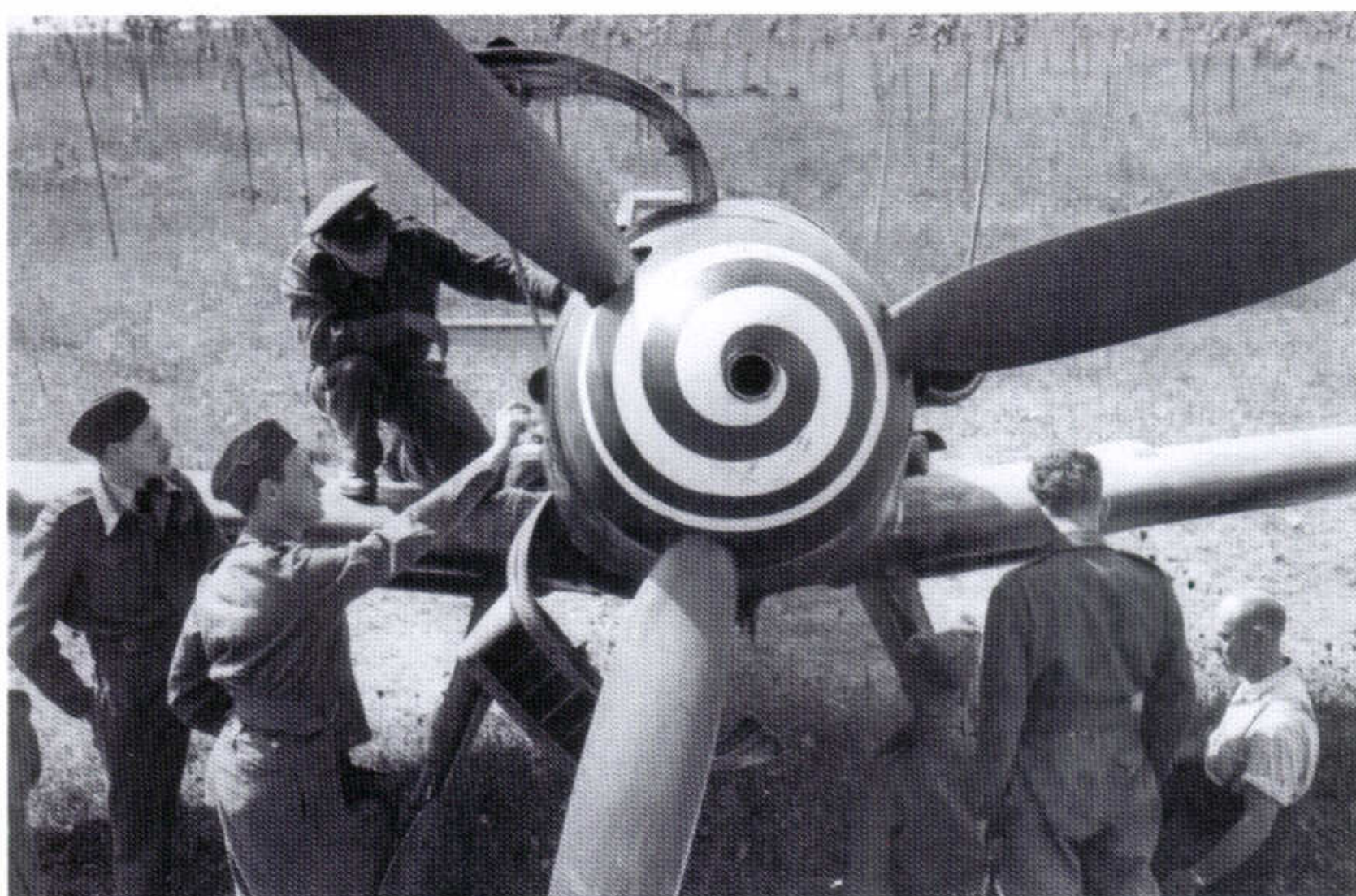
119: This Messerschmitt Bf 109 in RAF hands offers a classic view of the identification spiral applied to Luftwaffe fighters. Note, however, that the blade roots do not have the natural metal portion used to allow checking for blade alignment, but are overall RLM 70
