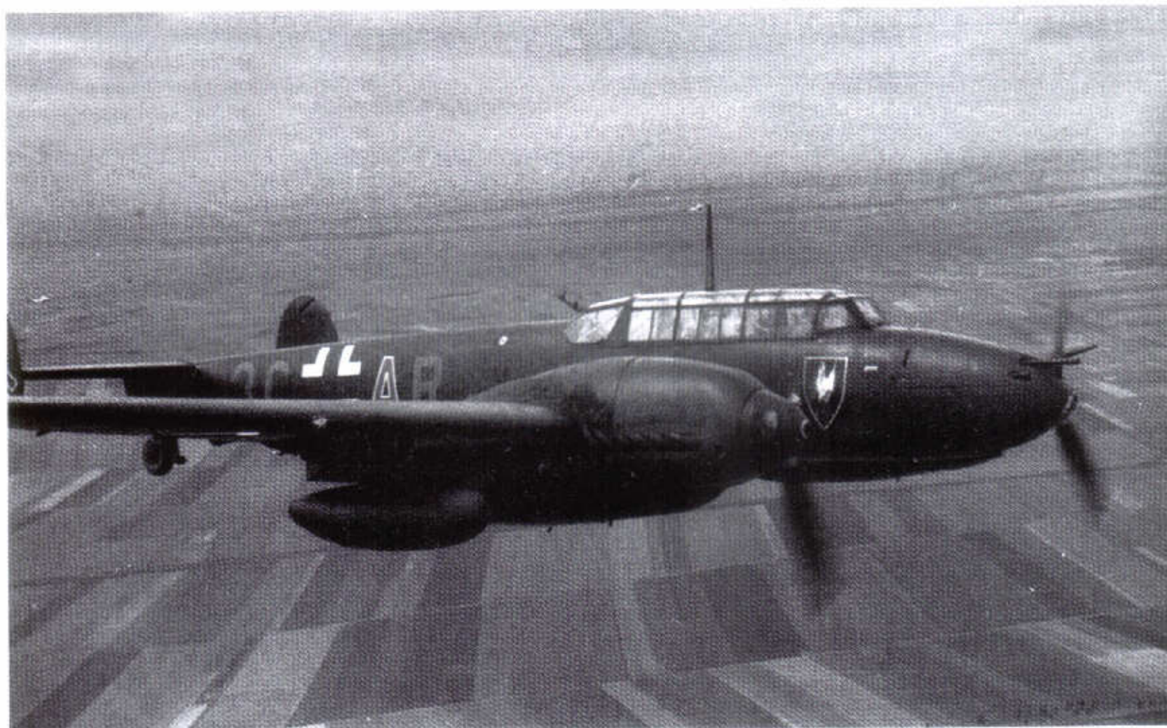
231: Oblt Kamp, staffelkapitän of 7./NJG 4 and his Bf 110E-4, 3C+AR, during a transit flight in 1942. Finished is the permanent 7124.22 black paint. According to regulations the code letters should be 77 but appear too dark. The cross should also be 77 (see page 225-226) but it is obvious that it is white, while the letters could be a dark grey or possibly red
