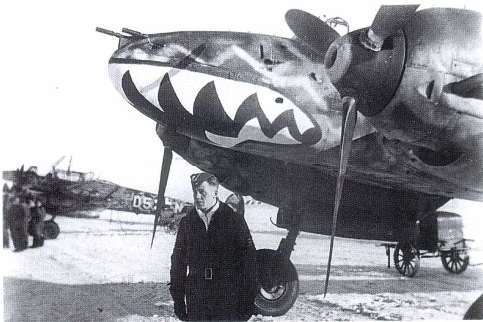
234 Above: Ju 88R-1, WNr 360043, D5+EV, in British markings. The aircraft has a 70/71/65 finish with over-painted German markings. The sharp colour demarcations line between the 65 and the upper camouflage colors is a sign of careful application of the paint, giving the expensive aircraft very good surface protection
