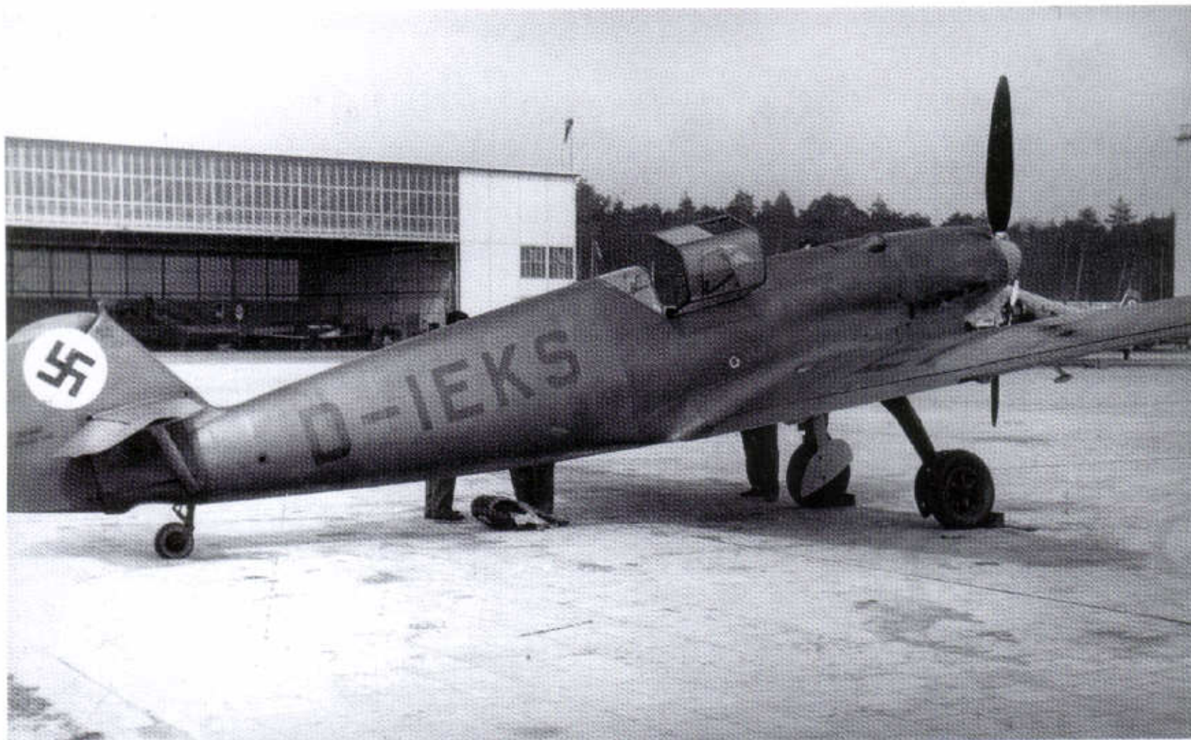
48: This is the Messerschmitt Bf 109V-5 (B-02) in 1936, fitted with a variable-pitch VDM propeller. It was later sent for trials with the Legion Condor in Spain. Here it wears a Class B1 civilian registration, D-IEKS, on what appears to be low contrast camouflage of RLM 70/71, a portion of the pattern of which can be just made out on the nose below and diagonally forward of the air intake. The spinner appears to be light grey or yellow. While the serial number for this aircraft is recorded elsewhere as 879, the legend 'WNR 320' can be made out on top of the fin in the original photo
