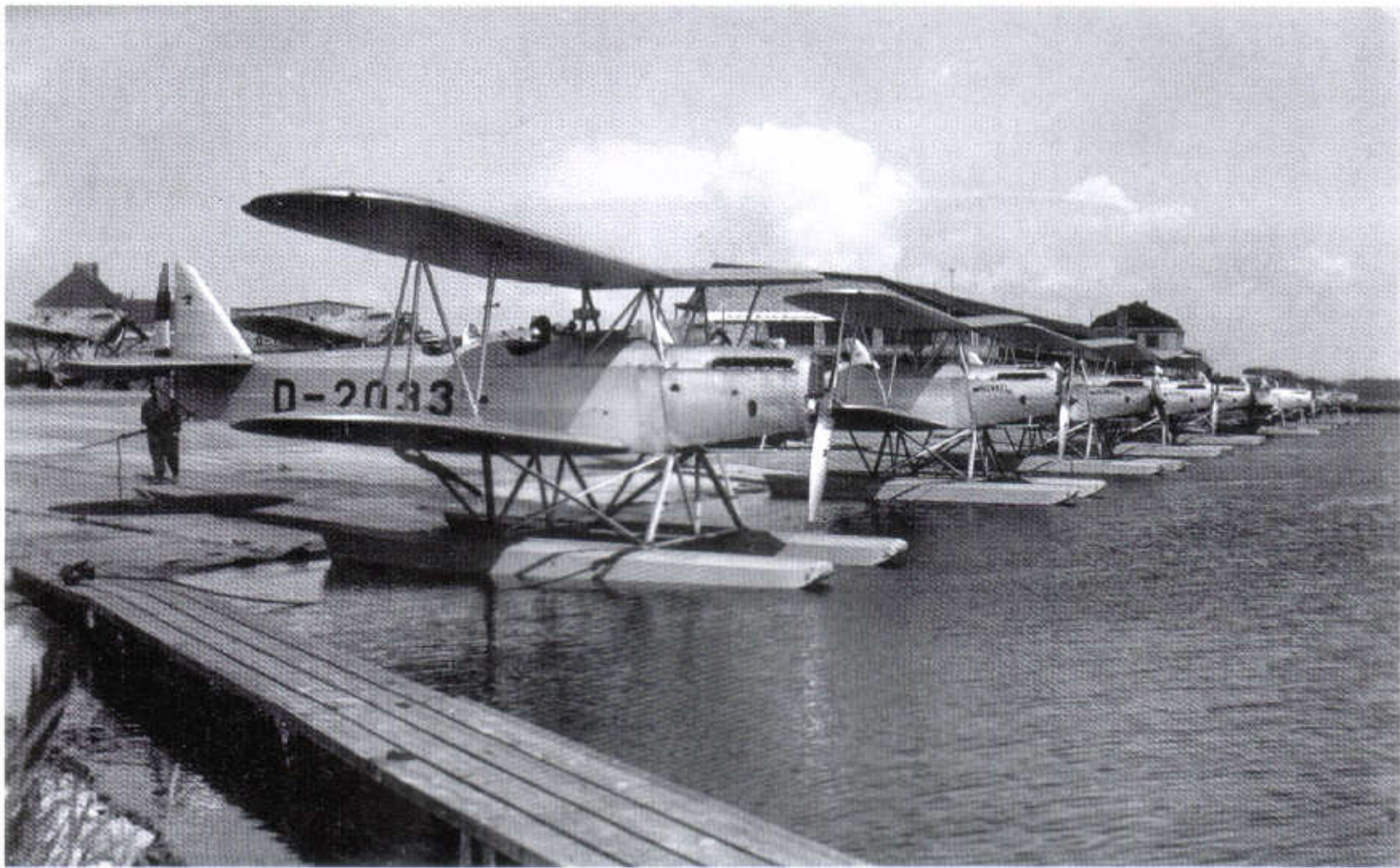
160: A line of Heinkel He 42B training floatplanes in Silber 01 drawn up on the slipway at Warnemünde. Civil registrations are in accordance with the regulations of the time which pre-date the Nazi era (see page 144). D-2033, the nearest machine was first registered in April 1931 to the DVS. This machine certainly survived until at least 1934. Note the small winged 'H' Heinkel trademark on the fin. The two aircraft just visible in the background are Heinkel He 9 monoplane floatplanes, world record holders in their day (AMC)
