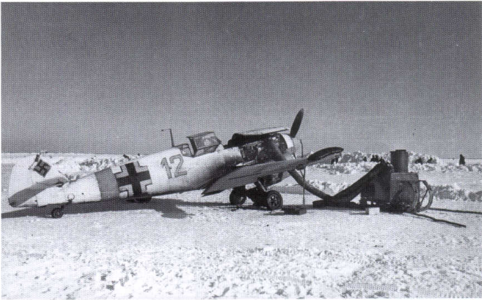
199: 'Yellow 12', a Bf 109F-2 of 3./JG 51 on the Eastern Front has received temporary white camouflage applied by brush, as per instructions, carefully avoiding the swastika and yellow theatre band. Contrary to regulations, however, the upperwing Balkenkreuz have been obscured. Note the warm-air blower on a sledge, needed to pre-warm the engine before it could be started
