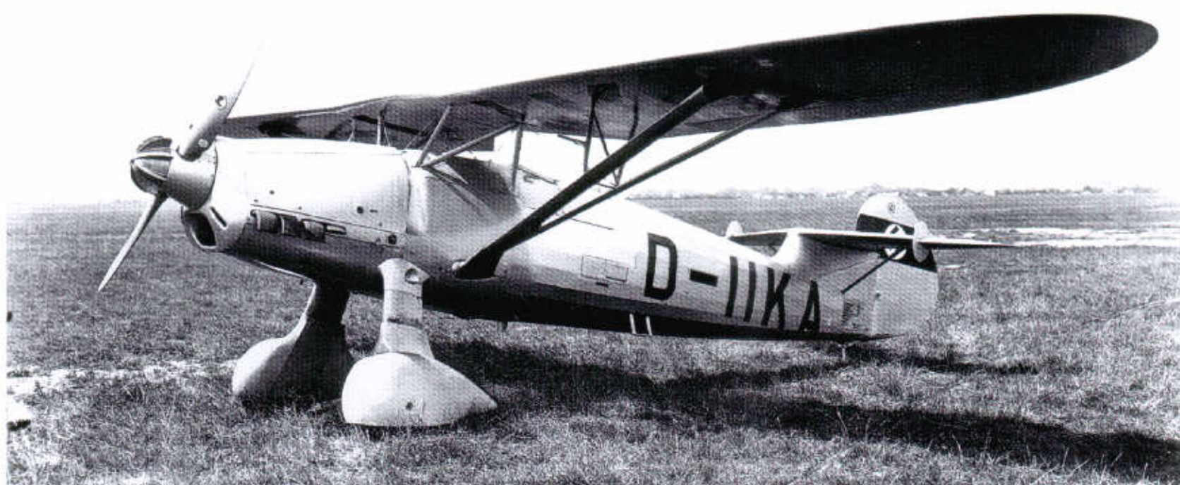
283: The Focke-Wulf Fw 56V-2 wears the standard civilian markings of early 1934, shortly after letter registrations had come into effect. At this time the swastika was only applied to the port side of the fin and rudder. Note the data table under the tail strut giving details of weights and limitations. Finished in overall silver, the aircraft had a vaned propeller spinner fitted in connection with dive-bombing trials
