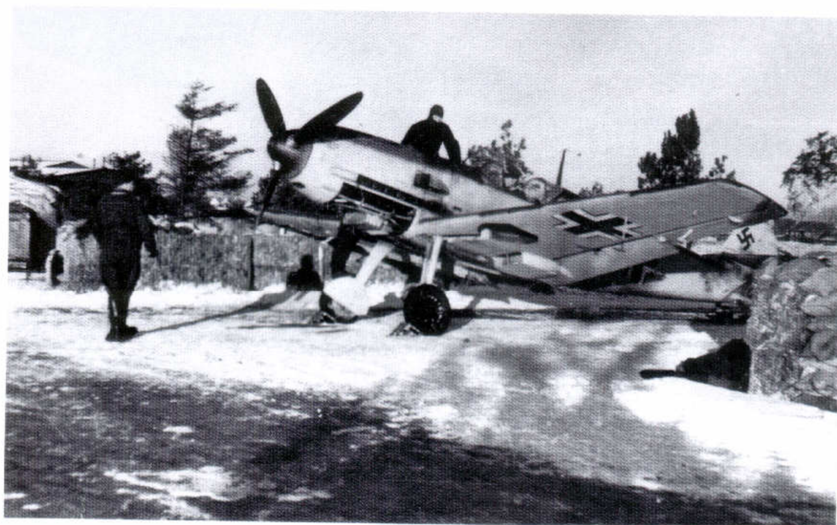
76: A Bf 109 E-1, believed to belong to II(J)/186(T), at Nordholz in Germany in winter 1939-40. Camouflage appears to be 70/71 or possibly 02 with 65 fuselage sides. This may have been applied at unit level as the swastika has a white frame but no visible thin black border. The underwing Balkenkreuz has the thin black border
