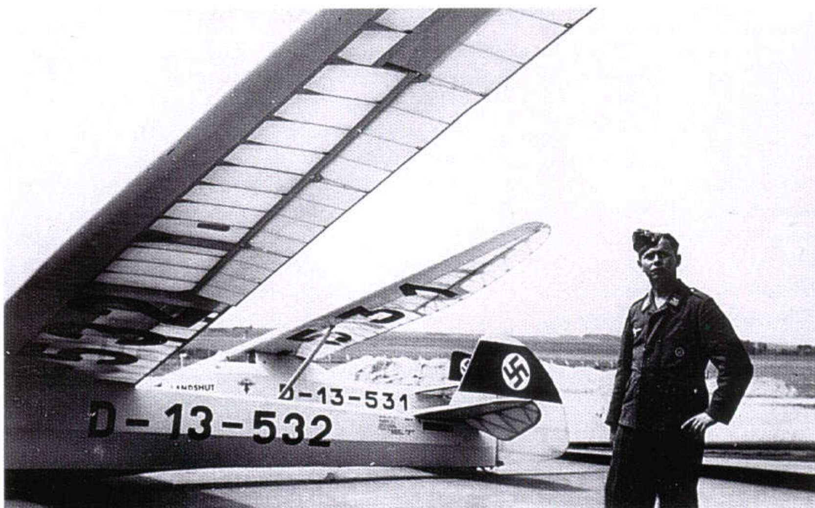
249: 'D-13-532' identifies this glider as a München Milan (?) in service with district 13 (Nuremberg) of the NSFK. It is painted in a clear lacquer on the wings and a light colour on the fuselage, probably a pale cream. It should be noted that the NSFK pre-war had its own colours, numbered FAS 1 to FAS 6. FAS 1 was a pale cream, lighter than RLM 05, and close but not identical to, modern RAL 1015. All markings are in conformity with official requirements. 'D-13-531' is a Göppingen Gö 1 Wolf. It carries the NSFK emblem on the fuselage below the cockpit
