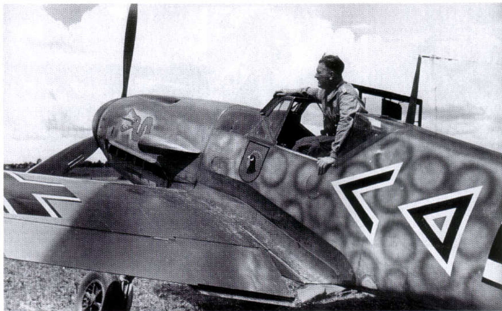
93: JG 3 also had some unusual ideas about camouflage. This Bf 109F of the Geschwader Kommodore, Major Hans von Hahn, has acquired circles of RLM 74 or possibly a dark green over the original 76 on the fuselage sides. The dark tone has also been brought up from the wing root onto the fuselage, probably in order to disguise exhaust staining. The command markings are also non-standard, the triangle being a unit-level invention. Note the much lighter tone of the 75 grey on the wing compared to that on the fuselage, and the early-style wing Balkenkreuz
