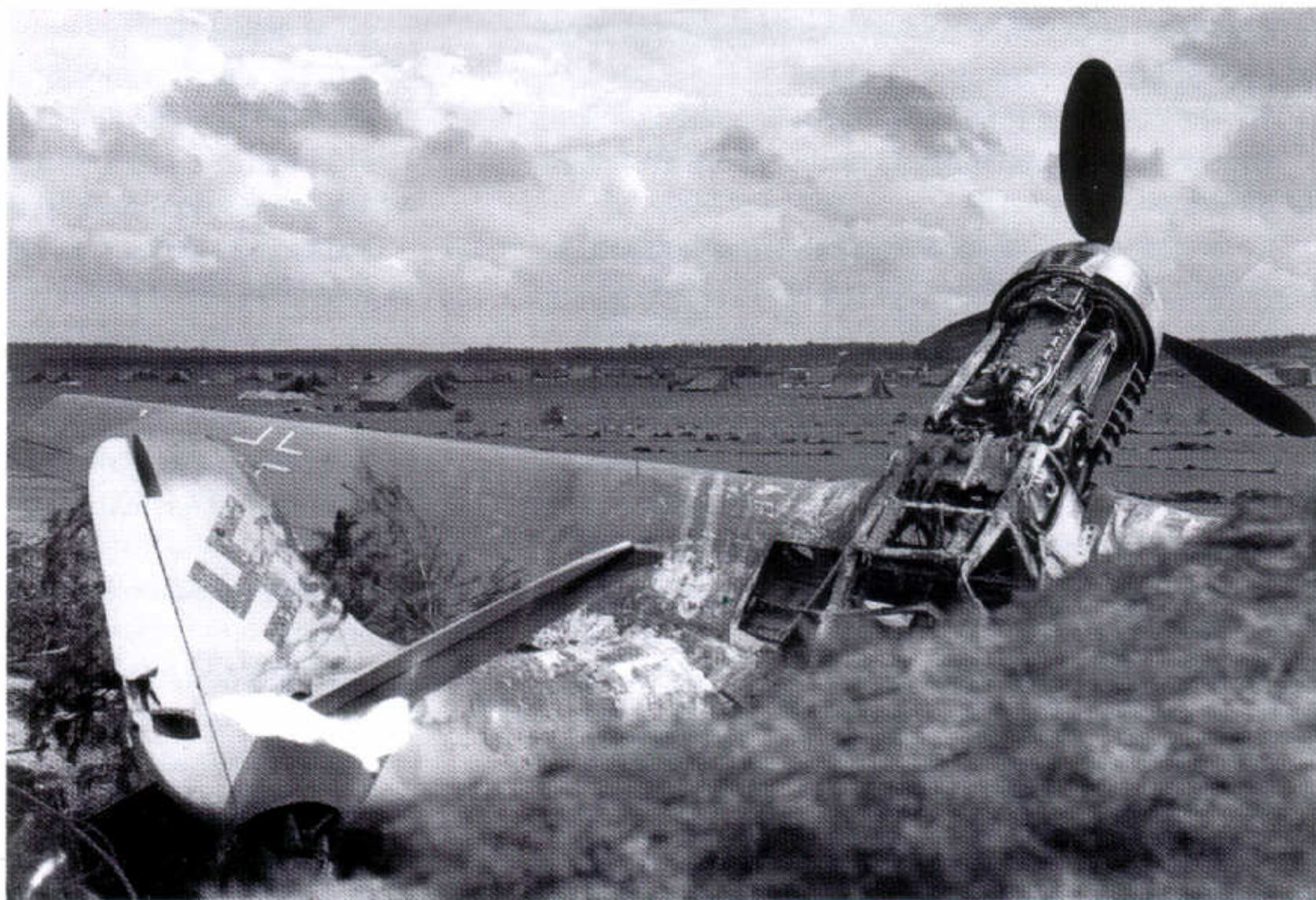
351: The wreckage of a Ta 152H of Stab./JG 301, destroyed by its last owners on the airfield at Leck. The wings show the camouflage pattern well, the colours being 81/82. The very pale tone, almost white, of the 76 on the fin is obvious, while the enormous paddle-bladed propeller and the small vents on the cowling are notable details
