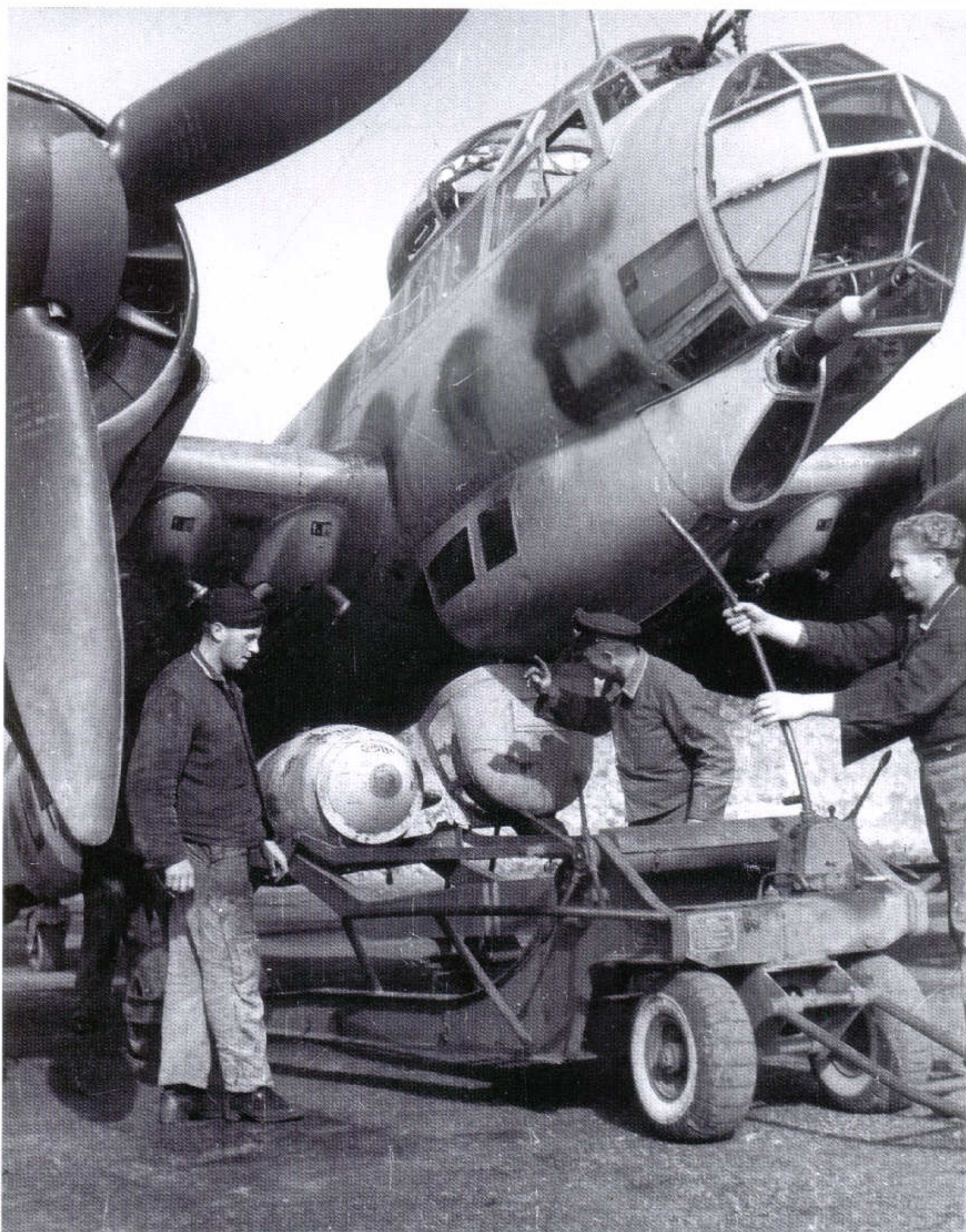
151: A Ju 88A-14 of LG 1 operating from Tunis in 1943 in tropical camouflage 79/78 with blotches of 80. One third of the spinner is painted in red 22 or green 25. An interesting detail on the propeller blades is the technical data and the wearing away of the paint on the leading edge. Both the white fuselage theatre band and the nose-mounted 20mm cannon are visible.
