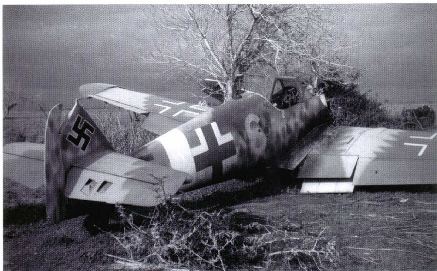
157: Towards the end, there was no time to apply tropical camouflage. This Bf 109G, 'Yellow 6', possibly at Anzio in Italy, still wears 74/75/76. The camouflage on the wings and tail is sprayed over masks with an unusual 'sawtooth' edge. This is clearly a misinterpretation of the rules directing merging of the edges between colours. The swastika lacks the black border, while the Balkenkreuz are the most simplified form, that on the fuselage being infilled with a dark tone, possibly 71, as it looks much darker than the 74 on the wings. Note the remains of a transit code ending in 'YY'
