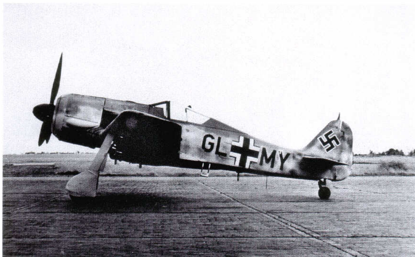
296: A factory-fresh Fw 190A-4 wearing a typical Stammkennzeichen delivery code on its 74/75/76 camouflage. All markings are typical for a fighter aircraft produced in the first half of the war
