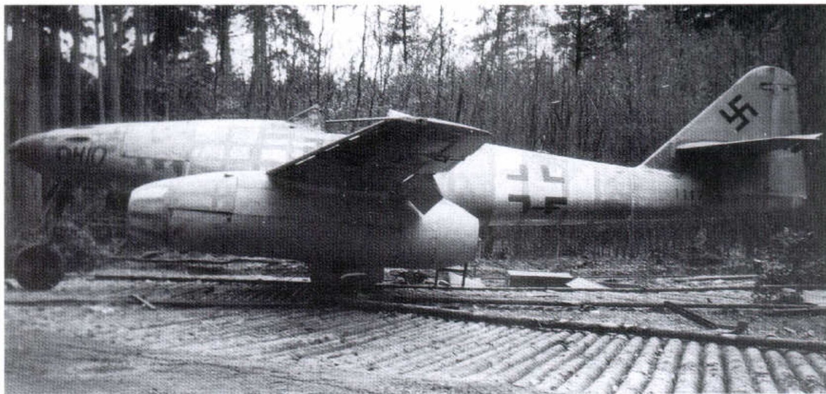
331: An unpainted Me 262 from the closing weeks of the war is a perfect example of the surface preparation of fighters late in the war. Compare the photo with the finishing instructions for the BV 155 on page 193 and the note concerning surface putty on page 209. It is clear that every panel line was filled and sanded. The aircraft has the maximum simplified national insignia. The position of the Werknummer, 111759, is unusual
