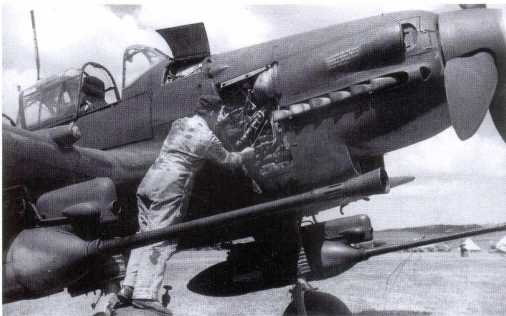
106: A fitter attending to the engine of a Junkers Ju 87G-1 tank-hunter. Although the official scheme was for the classic RLM 70/71/65, the aircraft shows signs of re-painting around the stenciling on the air intake which may indicate that it is now one overall colour. A spinner ring in yellow(?) the staffel colour, can be just made out. The completely matt finish is worthy of note
