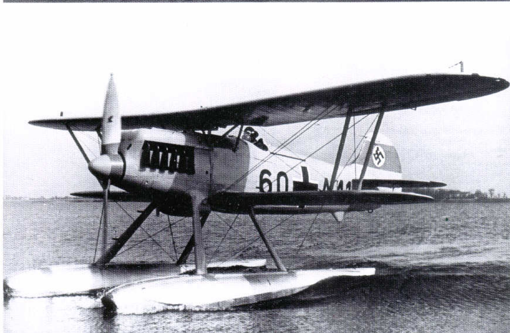
165: A photo of the very rare Heinkel He 51B-2 with floats. The aircraft was painted in the pre-war light grey L40/52, while the floats received a final coat of Silber 01 for maximum protection. All markings date from the 1936 period, the '60+A11' code indicating that the machine, 'A', is in service with 1/Küstenjagdgruppe 136, based at Kiel-Holtenau in late 1936. Note the manufacturer's trade mark on the propeller blade
