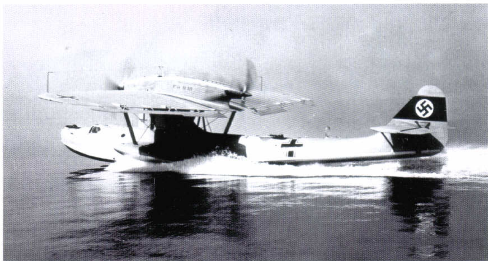
163 Above: Dornier Do 16 Wal D-ABAU, the militarised version of the Dornier Do J IIc, with a cover civilian registration belonging to the Seeflieger staffel based at List, about 1935, probably in L40/52 Grau finish above the waterline. The wings may be 04 Gelb
